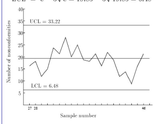
Number of defects in samples of 100 printed circuit boards
