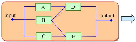
$$R_{sys}(t) = R_{sys}(t \mid B)R_{B}(t) + R_{sys}(t \mid \overline{B})(1 - R_{B}(t))$$
